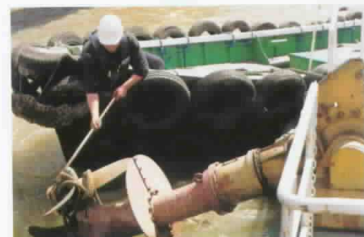
NO DRY DOCKING – Crewman removing rope fouling the propeller after elevating the transmission
